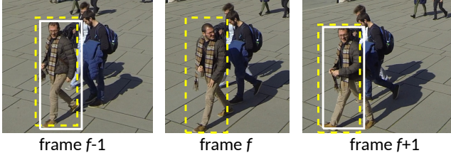
Figure 4: Illustration of Positives Mining. The solid white boxes denote detections, and the dashed yellow boxes are associated with the tracking algorithm.
